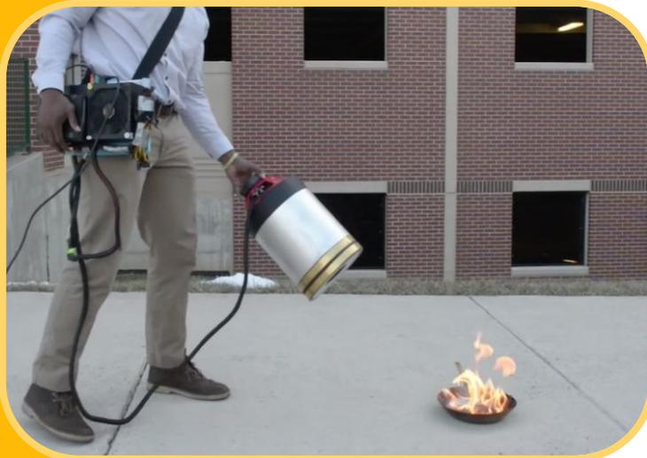
**Two engineering students from George Mason University have invented a new fire extinguisher, capable of putting out flames by manipulating sound waves.**
